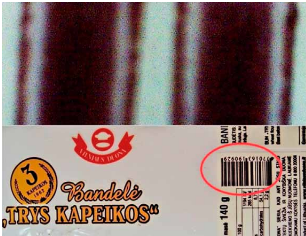
3 pav. Perspaudimas Fig. 3. Not adequate pressing force
