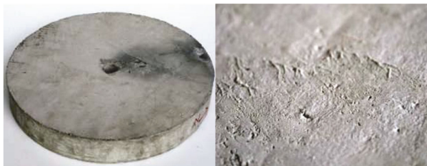
Smooth Portland cement concrete sample
