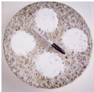
Fig. 2. Volumetric sand patch tests performed on an exposed aggregate concrete sample
