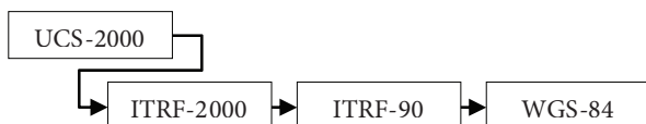
Figure 3. Scheme of coordinate transformation from UCS-2000 to the old realization of WGS 84
