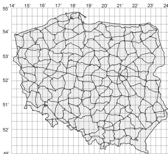
Fig 8. The grid of meridians and parallels 20' \times 20' against the background of Poland's borders and the double levelling network
