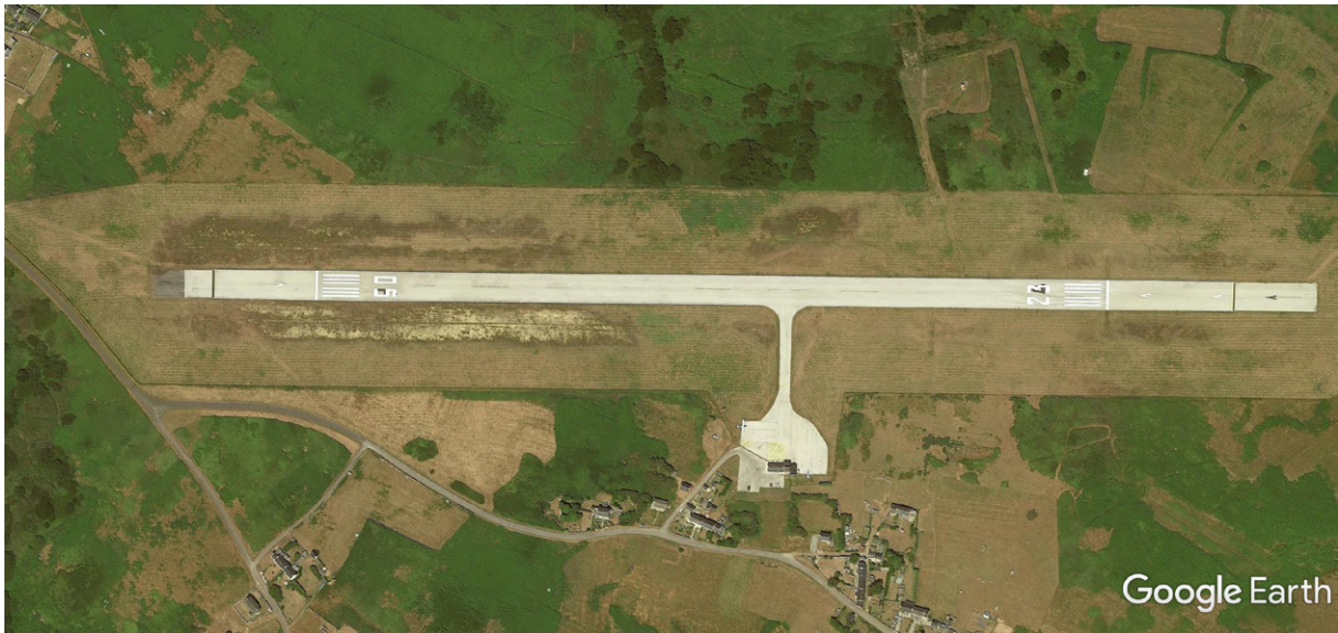
Figure 2. Aerial view of Ouessant airport. The runway is non-precision instrument runway. There is no approach light system, but low intensity edge lights and a PAPI. Strip width is 75 m
