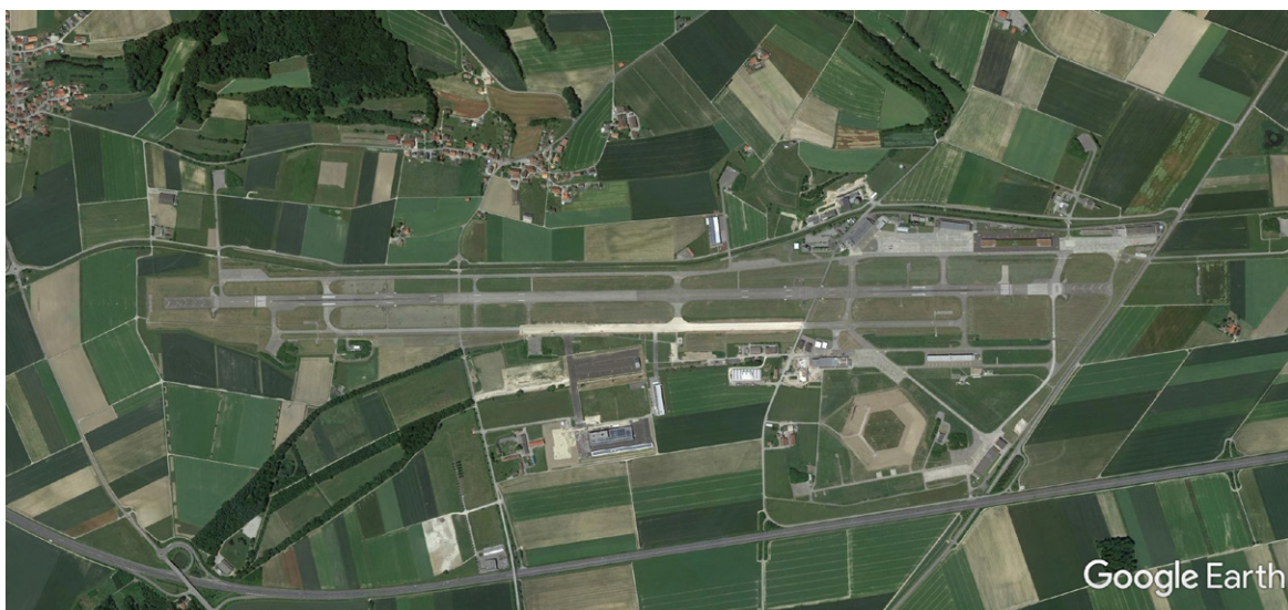
Figure 1. Aerial view of Payerne airport. The runway is classified as non-instrument. We can see the narrow width of the runway strip but also the CAT1 approach lights to either side. Arresting cables provisions are visible 450 m from threshold 0.5 and 750 m from the threshold 23. Strip width is 75 m
